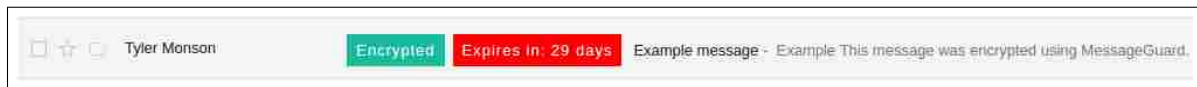
Figure 4.14: Labels for threads protected by an unexpired short-lived key show how long until the thread expires.
